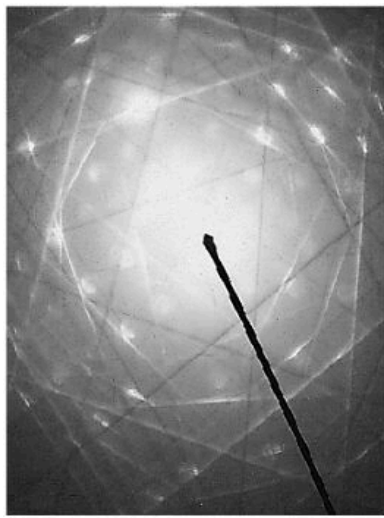
Transmission Kikuchi Pattern TEM, 250 kV
